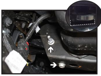
Using a 18MM socket & wrench, remove the two (2) bolts from the tow hook.
