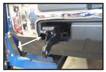
Slide the baseplate into the frame thru the tow hook pocket. Do this on both sides of the vehicle.
